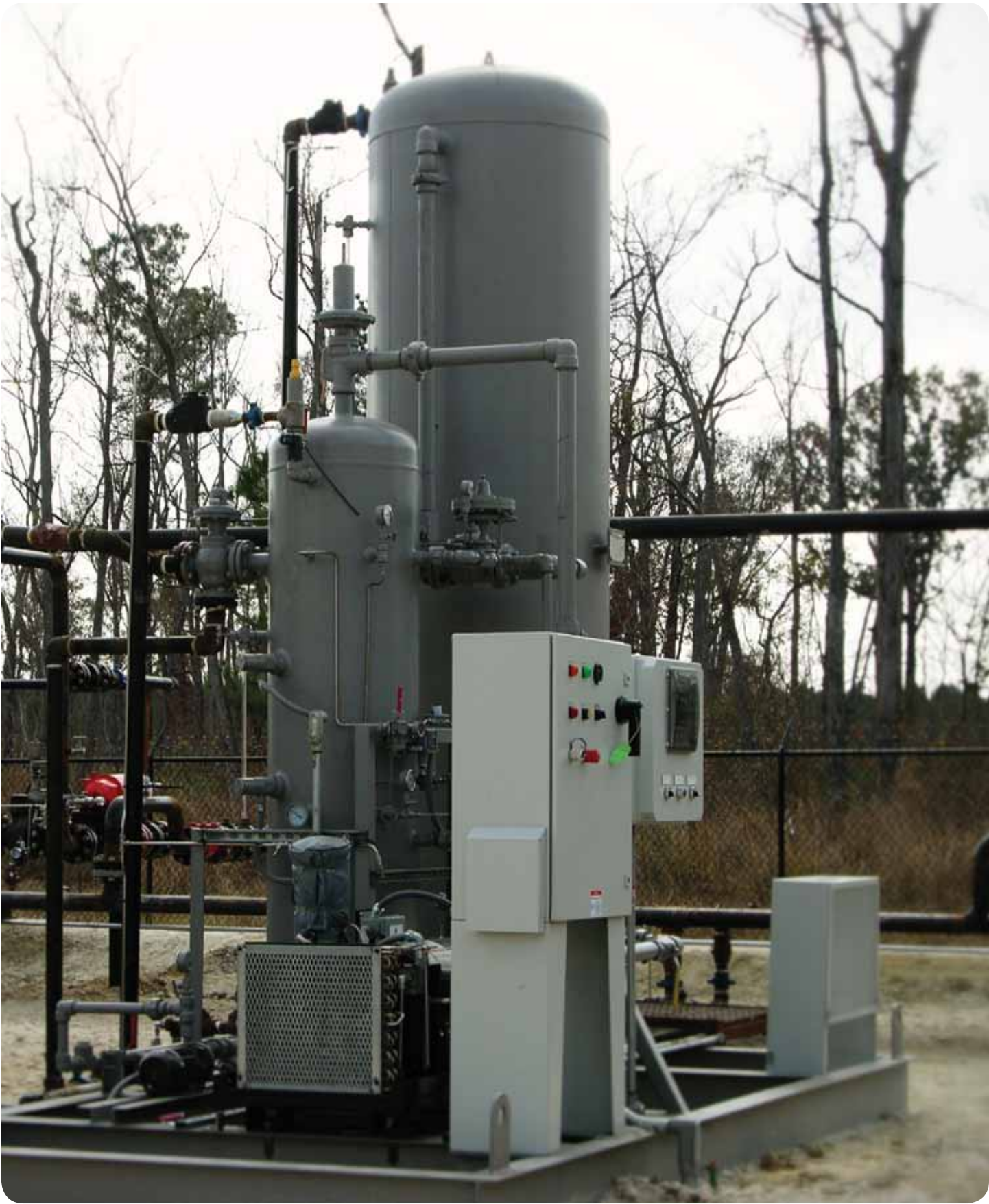
A portable short profile 300 barrel per day VRT/VRU package employs an electric pump to reduce tower height.
